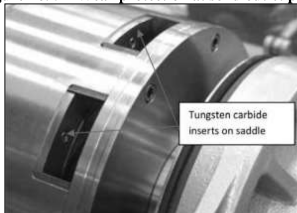
Figure no. 5 – Wear protection at solid outlet ports.
