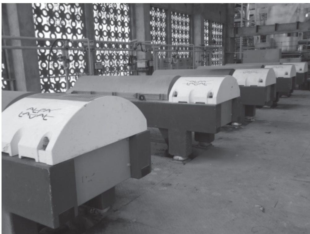
5 nos. SugarDec 400 decaners at Bannari Amman Sugars Ltd.
