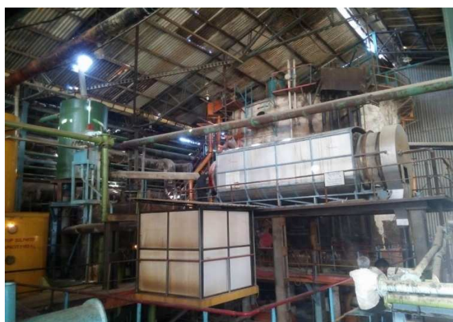
Fig 2. The hot raw juice RJS with gravity flow return at Sonhira factory.
