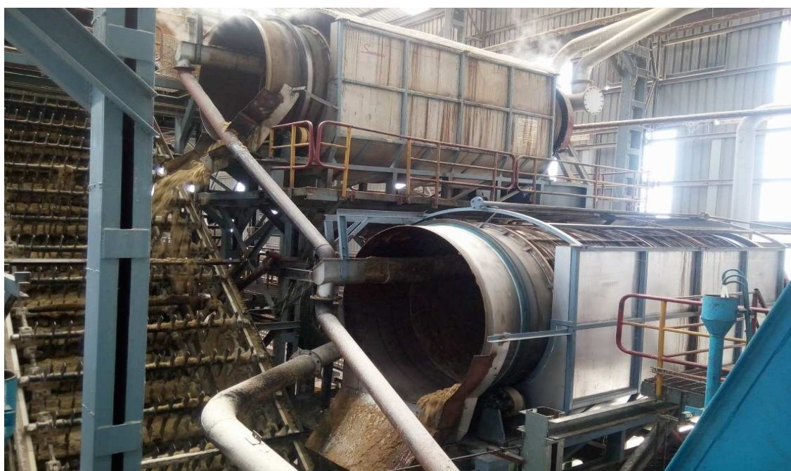
Fig 1. Two-stage RJS installation at a milling tandem of a 5000 tonnes of cane per day plant.
