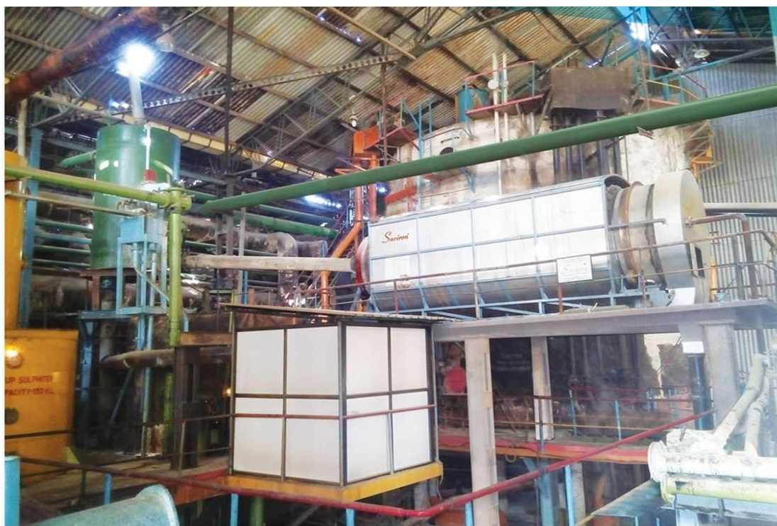
Figure no. 2 Installation of Rotary Screen for hot raw juice screening
