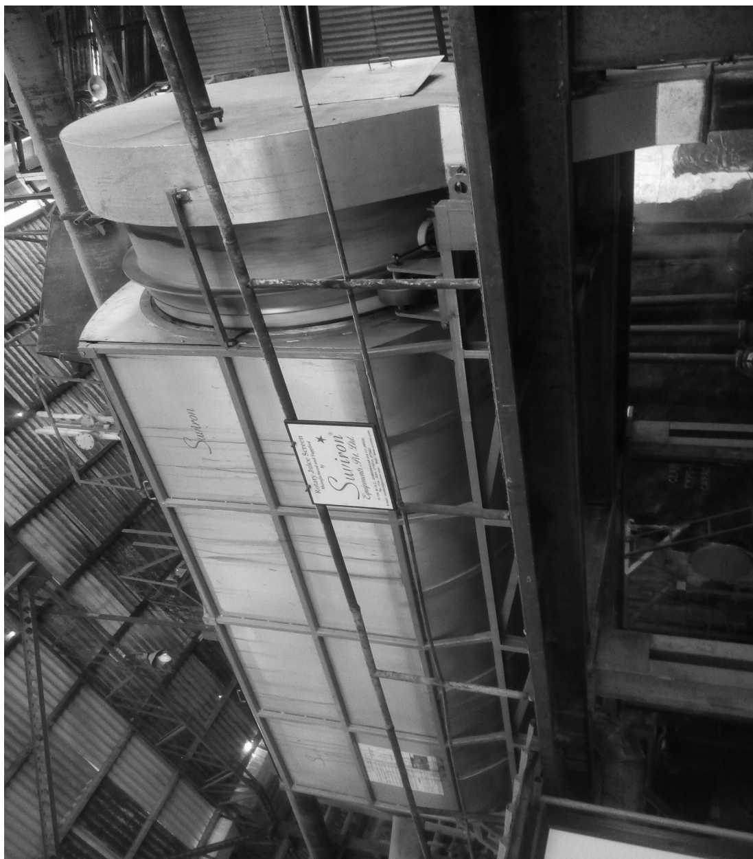
FIGURE 2 – INSTALLATION OF TOTALLY CLOSED ROTARY SCREEN FOR HOT RAW JUICE SCREENING
