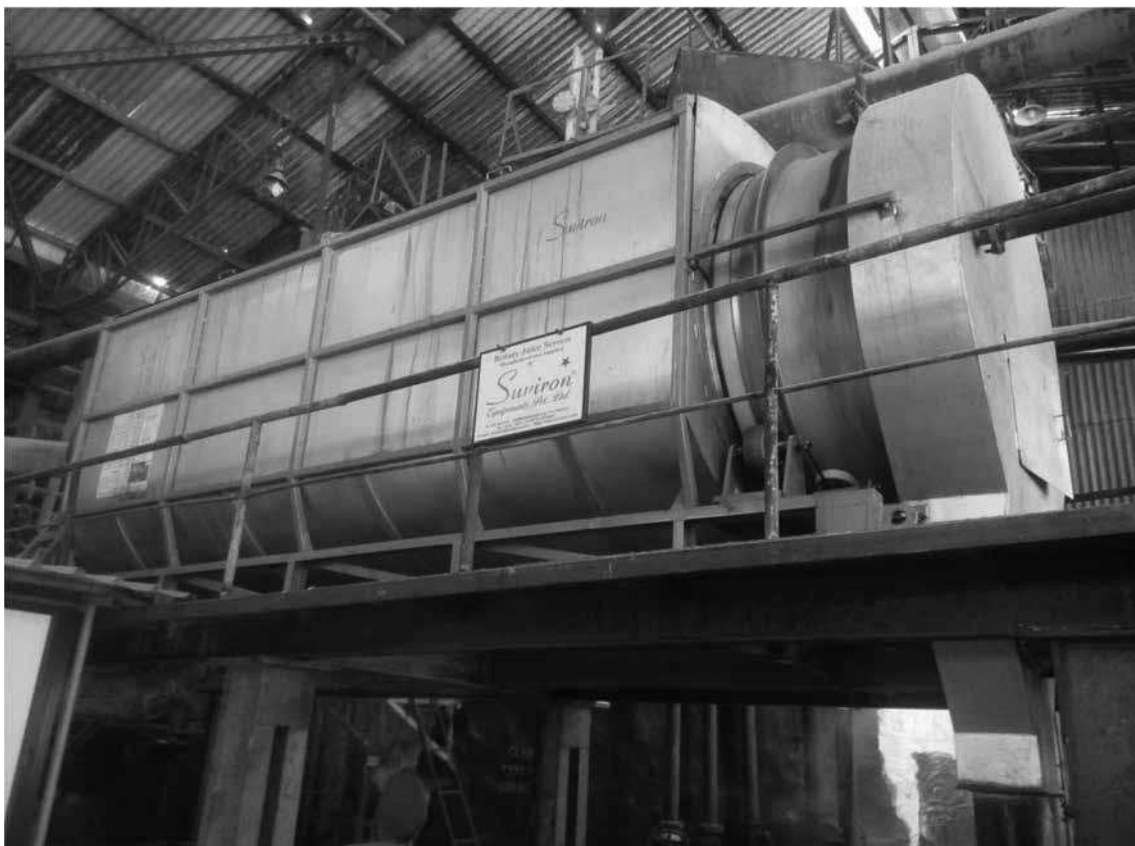
Totally closed Rotary Screen for hot raw juice screening
